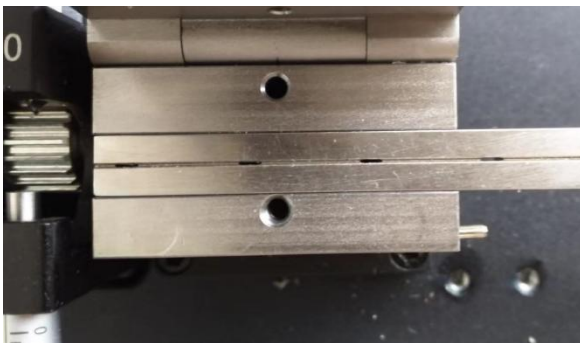
Different fiber holder adapters for different cladding diameter fibers (80~1250 \mu m)
